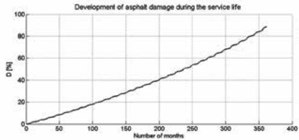
Figure 5b: Accumulation of damage during runway 14/32 service life
